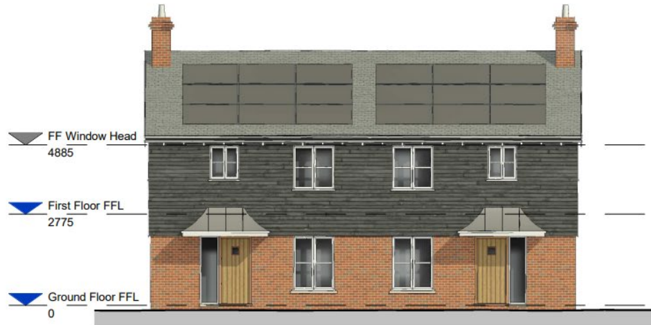
① Front Elevation 1 : 100
