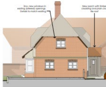
House 2 (Crocketts) - South Elevation as Proposed 1 : 100
