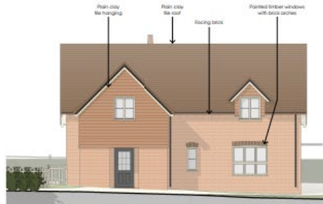
House 1 - West Elevation 1:100
